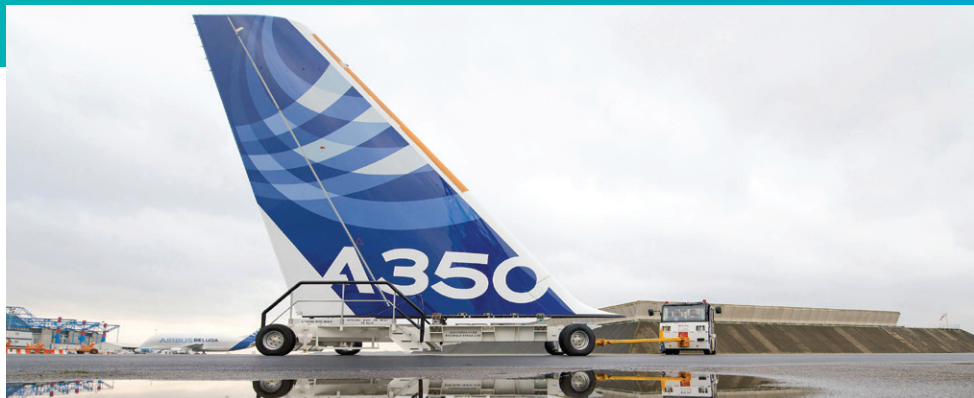
The 10-meter tall, composite vertical tail plane of the first A3 50 XWB that will fly (MSN1) has just come out of the paint hall in Toulouse wearing the well-known Airbus blue and white livery. The vertical tail plane is produced at Airbus' Stade site in Germany. Photo Credit: AIRBUS S.A.S. 2012 Photo by e'm company / H.GOUSSÉ.
