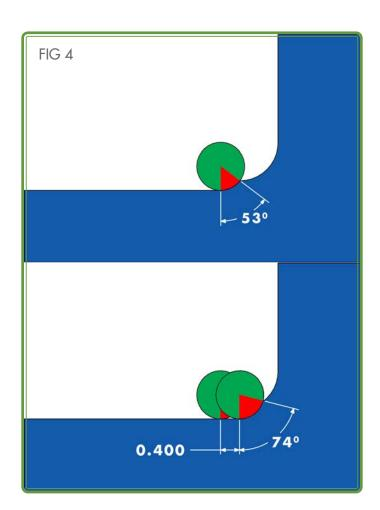
boundary, as established by the previous cut, to when the center of the cutter is normal to the same point on the current cut, a short span indeed. This dynamic is in play because of the concentric-natured construction of toolpaths: Whenever arcs are offset from one another in successive cuts within a toolpath, they are concentric with each other. It is this geometric configuration that ensures that this spike in tool load is ever present.
