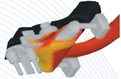
Metal front progression around a core
