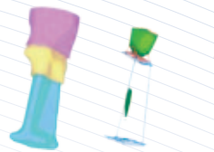
Initial wrapping design (left) and associated porosity (right)
