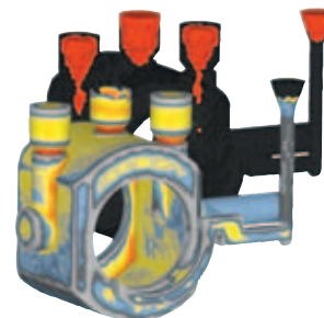
Pipe Shrinkage prediction for a steel component
